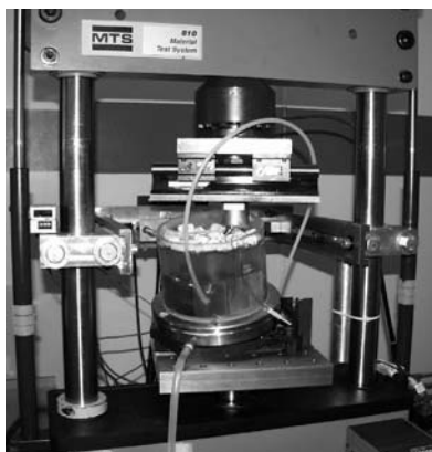
FIGURE 10 | Typical 10/9 Fatigue Testing Set-up with Environmental Chamber.
