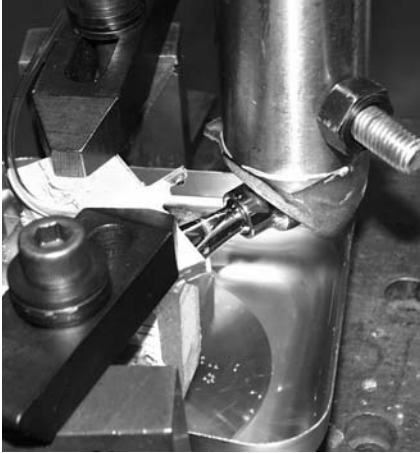
FIGURE 11 | Deep Flexion Testing Set-up with Saline Drip Over Neck Taper.
